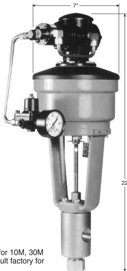
Remote Valve Stem Positioner "RVP" above permits remote positioning of valve stem in increments of 0.0112". To order, add suffix "RVP" to base order number.
